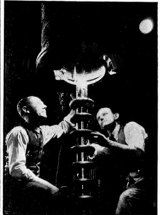
L. E. Dempster and W. F. Westendrop, assembling a million volt x-ray equipment. A novel feature of the construction is that the tube is enclosed in the center of the transformer, and that the equipment is small enough for installation in existing hospitals.
