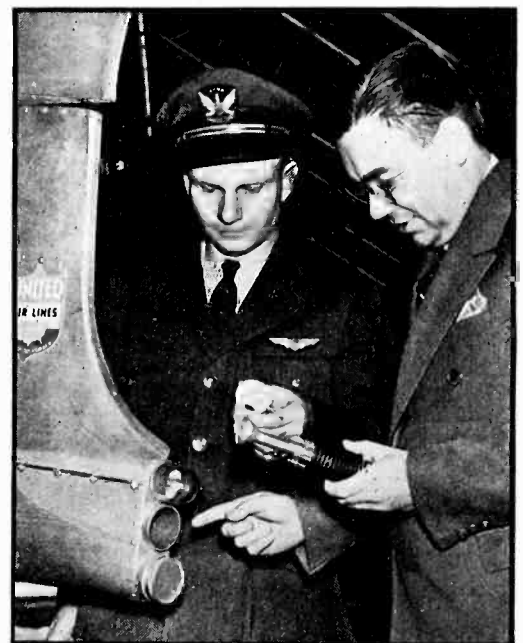
Static suppressor device, which when released from the tail of an airplane prevents static discharges from the plane surfaces
